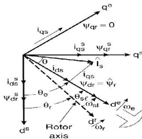
**Figure 3: Phasor Representation of Indirect Vector Control IM.**
