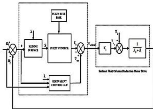
**Figure 2: Schematic of Fuzzy Sliding Mode Controller.**
