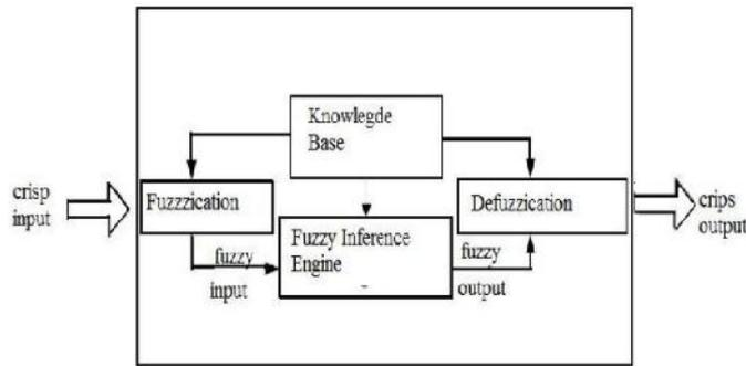
**Figure 4: Shows a Block Diagram of a Fuzzy Inference System with Logical Controller Consists of Four Basic Major Components: Defuzzification Fuzzy, Fuzzy Inference Engine and Knowledge Base.**
