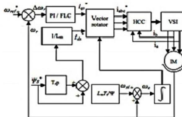
**Figure 1: Speed Control of IM Using Indirect Vector Control.**
